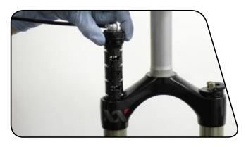
**15** Turn the damper clockwise to thread it into the upper tube. Be careful not to damage the damper top cap o-ring. Continue to thread the top cap down into the upper tube threads and hand tighten. Use a 24 mm flat wrench to tighten to 7.3 N·m (65 in-lb.)
