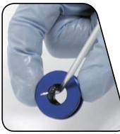
14 Re-install the top out bumper and negative piston onto the air shaft with the flat side of the negative piston oriented toward the air piston.
