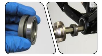
Press the bearing into bottom bracket shell until butted against the retaining clip. Repeat the process for the other bearing. Consult your headset press manufacturer's instructions for proper use of the headset press.
