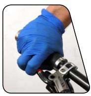
Once the large bubbles at the lever have stopped, apply a small amount of pressure on the syringe plunger then remove the syringe and re-install the bleed port screw.
