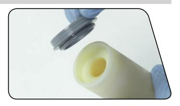
Hold one of the lower legs firmly and use the seal installation tool to push the dust wiper evenly and completely into that leg.
