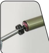
6 Slide the seal head off the damper shaft and use a pick to remove the inner and outer seal head o-rings. Apply a few drops of Pit-Stop suspension oil to new o-rings and install them.
