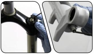
A Remove the external rebound adjuster by pulling it from the drive-side shaft bolt.
