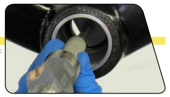
Removal of the retaining clips is unnecessary for bearing 5 replacement unless the retaining clips are damaged. The damaged retaining clip can be removed by using a flat bladed screwdriver to lift the notched section of the retaining clip out of the bottom bracket groove and guiding the retaining clip out of the bottom bracket groove.
