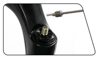
Use a 24 mm socket wrench to loosen and unthread the top cap. Remove the top cap and the entire air assembly from the top of the fork.
