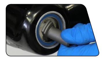
A Insert a driver (punch or drift) from the opposite side and place it against the back of the BB30 removal tool. Lightly tap the BB30 removal tool with a mallet until bearing is removed from the bottom bracket shell. Repeat for other side.
