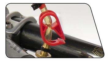
Pull out on the lever syringe plunger to create a vacuum, then gently push in on plunger to pressurize the system. Squeeze and release the brake lever ten times, allowing the lever to snap back to its starting position after squeezing (this helps break loose the bubbles). Repeat this procedure of creating a vacuum at the syringe and squeezing the brake lever ten times until large bubbles stop coming out of the lever.
