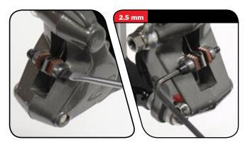
Remove the brake pads and spreader clip from the caliper and insert the appropriate Bleed Block. This will help prevent system overfill and keep DOT fluid from contaminating your brake pads.
