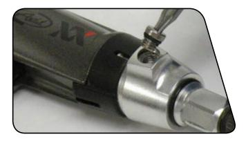
9 Make sure the fluid in the 1/4 full syringe is pushed all the way to the tip (no air gap!), then thread into the lever bleed port.
