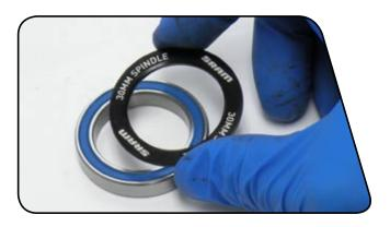
3 Apply grease to the inside surfaces of the bottom bracket shell, and the bottom bracket grooves. Apply light grease to the crank spindle splines and and spindle threads.
