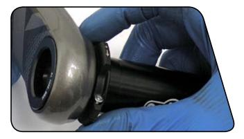
Install the bottom bracket cup seals into the bottom bracket cups. Slide the non-drive side crankarm spindle through the non-drive side bottom bracket cup until the splines come through the drive side bottom bracket cup, and the spindle stops. You may need to tap the crankarm with a rubber mallet to fully install the spindle into the bottom bracket.
