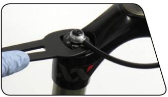
2 Remove the compression damper from the upper tube/crown by pulling up and rocking it from side to side. Once removed, clean the upper tube threads with a clean rag.
