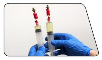
2 Take a moment to de-gas the fluid in the 1/2 full syringe. Leave the hose clamp shut and pull on the plunger. Bubbles will form in the brake fluid. While the plunger is still pulled down, lightly tap the syringe to release the bubbles sticking to the sides and the bottom so that they can rise to the top of the fluid. When the bubbles stop forming and have all risen to the top, release the plunger, open the clamp and carefully push the air out. Repeat several times.
