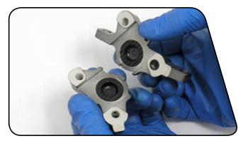
Using a sharp pick, remove the small banjo hole (body half) o-ring.
