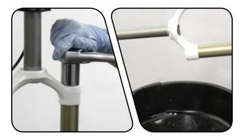
Clamp the fork back into the bicycle stand. Push the negative air shaft up and into base plate, leaving only the tip of the threaded shaft end protruding from base plate.
