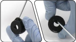
6 Re-install the base plate into the upper tube. Use large snap ring pliers to re-install the snap ring. Be sure to align the base plate tab between the snap ring eyelets. Apply a generous amount of grease to the base plate inner o-ring.
