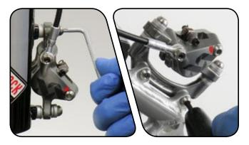
2 Use an 11 mm open ended wrench to hold the hose stop in place and use an 8 mm open ended wrench to unscrew the hose compression nut. Pull the brake hose and compression fitting from the brake lever body.
