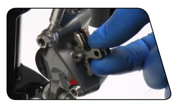
3 XX brake caliper pistons need to be pushed back into the caliper body before the new pads can be installed. Insert a large box-wrench (or similar tool without sharp edges) between the pistons, then carefully rock it back and forth, pushing the pistons back into their bores.
