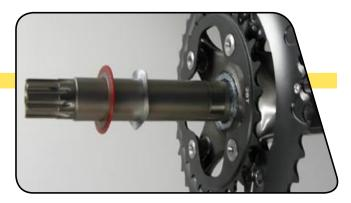
Slide the drive side crankarm spindle through the drive side bottom bracket cup until the splines come through the non-drive side bottom bracket cup, and the spindle stops.
