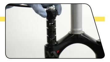
3 With a pick, remove the compression damper o-rings (located at the top and bottom of the damper). Apply a few drops of Pit-Stop suspension oil to new o-rings and install.
