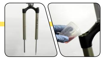
14 Insert the compression damper into the upper tube. Press down and rock the damper from side to side to work it into the upper tube.
