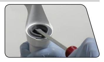
2 Stabilize the lower leg upright on a bench top or on the floor. Hold the lower leg firmly and use downward force on the tool handle to leverage the seal out. If your fork has an oil foam ring, remove it with your fingers.
