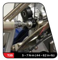
Attach the front/rear shifter cable to the front/rear derailleur. Make sure the cable follows all derailleur fins or guides, and is fully captured within the cable anchor plate.
