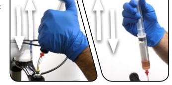
Unthread the syringe from the damper, and use a T10 TORX wrench to re-install the bleed screw into the damper. Use a rag to wipe off any excess suspension fluid.
