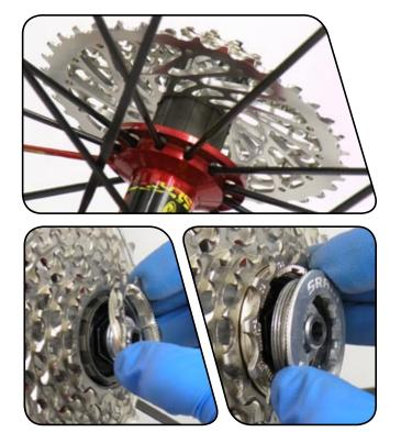
Use a freewheel tool (Park Tool\* FR-5 or equivalent) and a torque wrench to tighten the cassette lockring to 40 N·m (350 in-lb).
