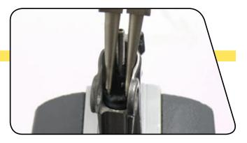
Replace the entire piston/bladder/snap ring assembly with a 9 new assembly. Lubricate the piston/bladder assembly by dipping it into DOT 5.1 fluid.
