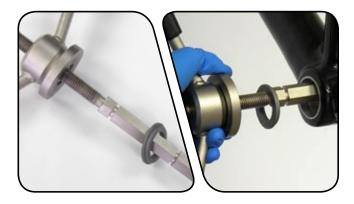
**6** Install a BB30 bearing onto the bearing installation part (with the blue seal facing the install part), and install the bearing installation part onto the headset press.
