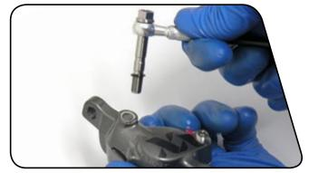
6 Use a T10 TORX to remove the bleed screw from the banjo bolt.
