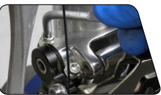
Click the small lever on the front shifter to ensure the cable is fully released. Turn the front shifter barrel adjuster fully into the shifter, then turn counterclockwise one full turn.
