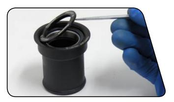
Apply grease to the bottom bracket and frame surfaces as illustrated, including the outside face of the bearings, and the drive side bottom bracket cup o-ring. Apply grease to the spindle threads, splines, and races (the smooth part of the spindle near the integrated preload adjuster).
