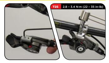
The lower shift lever is infinitely adjustable. Use a T25 TORX wrench to loosen the adjustment bolt. Position the shift lever to suit your ergonomic needs. Hand tighten the adjustment bolt.
