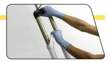
Invert the fork to about 45°, fork legs pointing upward. Measure and inject/pour 5 ml of 15 wt Pit-Stop suspension oil into lower legs through each shaft bolt hole, Wipe all excess oil from the lower legs.
