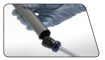
15 Use a pick to remove the air piston o-ring. Apply grease to the new o-ring and install it.
