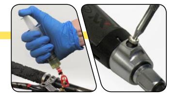
Spray isopropyl alcohol or water onto a towel and wipe off the brake lever and caliper to remove any excess DOT fluid.
