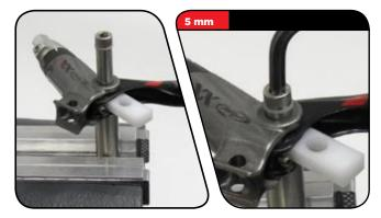
**5** Use a 2 mm hex wrench to turn the reach adjust pushrod clockwise until it unthreads from the pushrod pivot pin.
