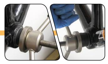
3 Install the wave washer and then the drive side bearing shield onto the spindle, making sure the bearing shield is oriented correctly. The stepped lip on the bearing shield should face the bottom bracket shell.
