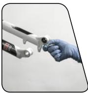
6 Firmly pull the lower leg downward until oil begins to drain.
