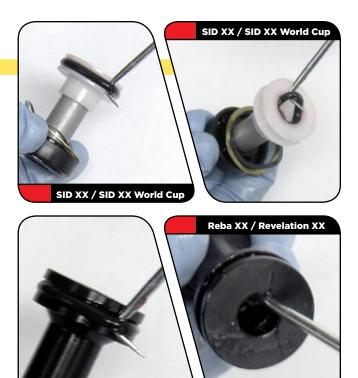
8 Use a pick to remove the air piston o-ring. Apply grease to the new o-ring and install it.
