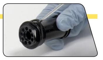
Use small external snap ring pliers to remove the small external snap ring located at the bottom of the air assembly, then remove the negative piston retention plate.
