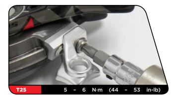
Install the MMX bracket nut on the inside surface of the MMX 2 clamp. Position the MMX bracket assembly on the outside of the MMX clamp and loosely install the MMX bracket bolt to hold the assembly in place. Use a T25 TORX wrench to torque the bracket bolt to 4 - 5 N·m (25-30 in-lb).
