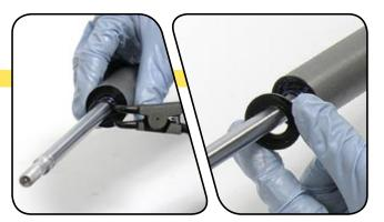
Use large internal snap ring pliers to remove the snap ring from 10 the bottom of the air tube. Use the tips of the pliers to press the aluminum negative piston slightly into the air tube while installing the snap ring for a more secure snap ring engagement. Remove the snap ring by guiding it off of the air shaft by hand.
