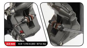
6 Install the pad retainer bolt and use a 2.5 mm hex wrench to torque to 0.9-1.1 N·m (80-97 in-lb). Install the "E" clip on the wheel side of the caliper making sure it sits in the groove of the retainer bolt.
