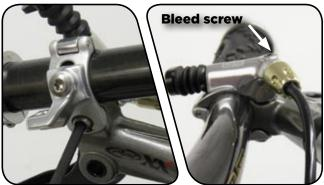
2 Use a T25 TORX wrench to loosen the XLoc handlebar clamp, position the XLoc so that the bleed screw is slightly above the button, and re-tighten the clamp bolt.
