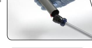
Wipe any remaining grease from the snap ring groove with a clean rag. Use large internal snap ring pliers to secure the snap ring into its groove.
