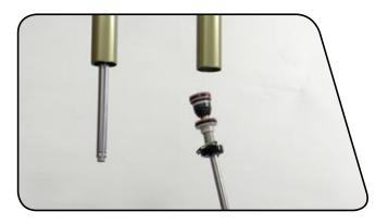
5 Spray isopropyl alcohol on the inside and outside of the upper tube and wipe with a clean rag. Wrap a clean rag around a long dowel and insert it into the upper tube to clean inside the upper tube.
