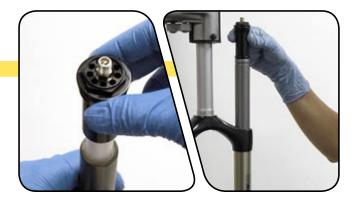
21 Apply a few drops of medium strength thread lock to the top cap outer threads. Use a 24 mm socket wrench to thread the top cap into the upper tube. Tighten it to 14.6 N·m (130 in-lb).
