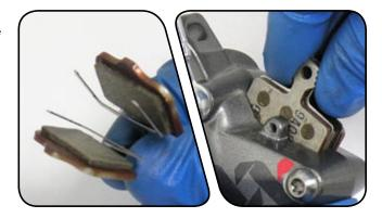
Using a 2.5 mm hex wrench, install the pad retainer bolt and tighten to 0.9-1.1 N·m (8-9.5 in-1b). Install the "E" clip on the wheel side of the caliper making sure it sits in the groove of the retainer bolt
