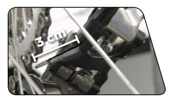
9 Feed the cable through the cable housing and stops. Make sure the rear shifter is in the fully released position (highest gear). Turn the barrel adjuster clockwise fully into the shifter, and then unthread one full turn.
