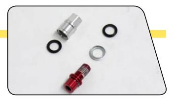
6 Insert the rebound damper and air spring shaft bolts into threaded shaft ends (or air shaft nut onto the threaded shaft end), through the lower leg shaft holes and tighten with a 5 mm hex or 10 mm socket wrench to 7.3 N·m (65 in-lb).
